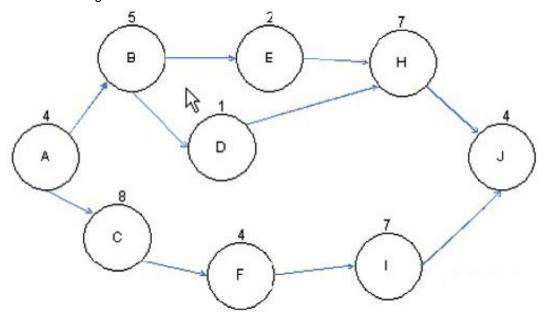
Based on the project network diagram, how much float is available for Activity H if Activity B is delayed by four days and Activity E is delayed by two days?
