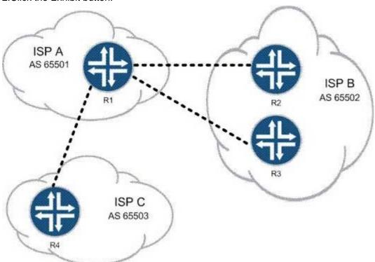
You work for ISP A. Customers of both ISP B and ISP C must be able to reach all of your customers, but your network must not allow transit traffic between ISP B and ISP C.
