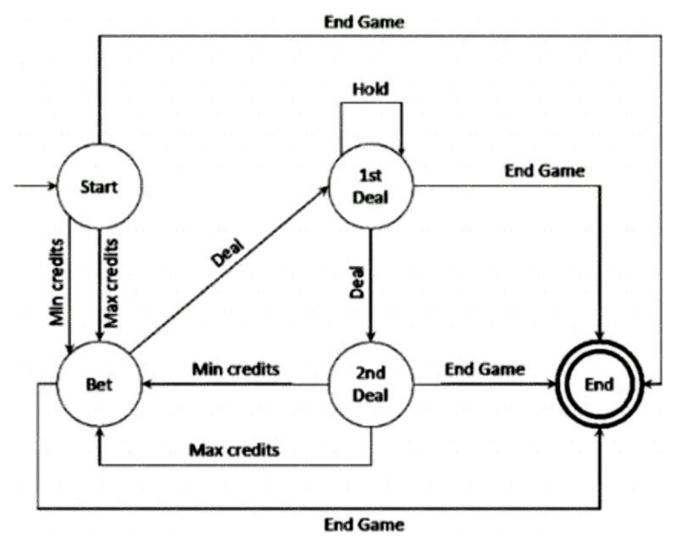
What Is the minimum number of test cases needed to cover every unique sequence of up to 3 states/2 transitions starting In the "Start" state and ending In the "End" state?
