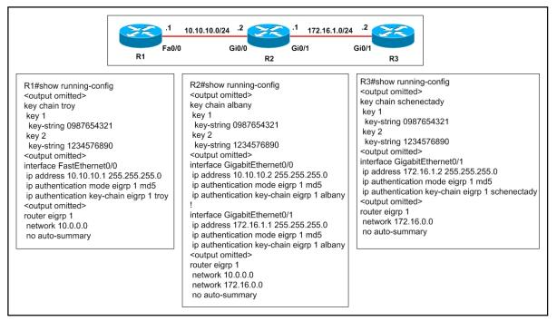
EIGRP is configured on all routers in the network. On the basis of the output provided, which statement is true?
