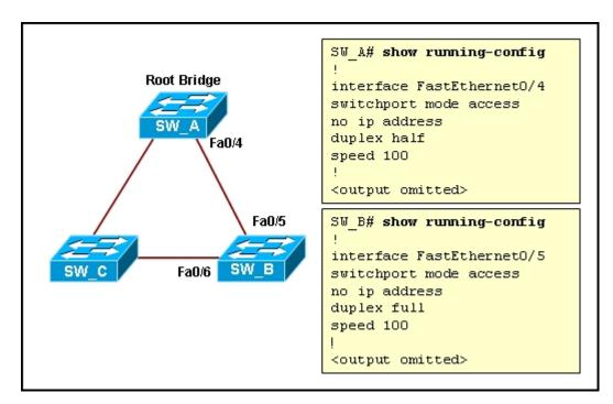
and the partial configuration of switch SW\_A and SW\_B. STP is configured on all switches in the network. SW B receives this error message on the console port:
