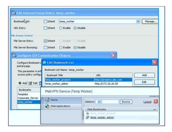
Refer to the exhibit. A new network engineer configured the ABC adaptive security appliance with two bookmarks for a new temporary employee. The temporary worker can connect to the administrator server via the temp\_worker\_admin bookmark but cannot connect to the project server via the temp\_worker\_projects (greyed-out) bookmark. It was determined that the URL and IP addressing information in the GUI screens is correct.
