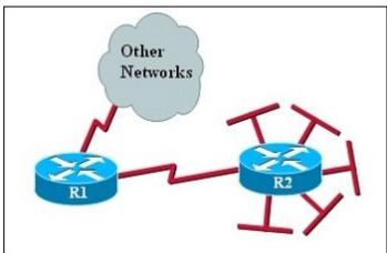
The networks connected to router R2 have been summarized as a 192.168.176.0/21 route and sent to R1.
