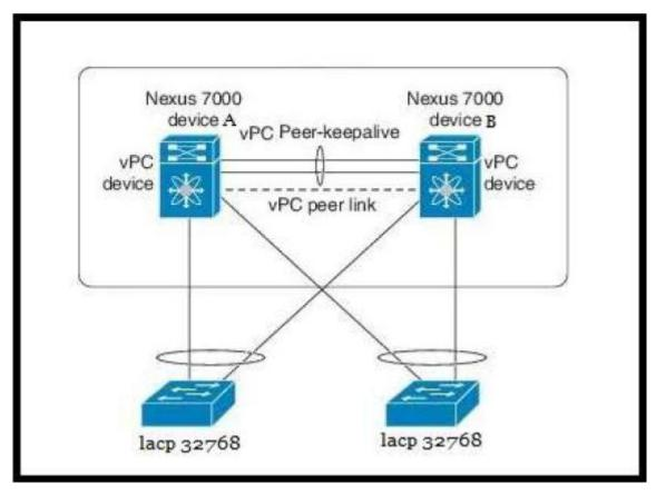
Which configuration ensure that the cisco Nexus 7000 series switches are the primary devices for LACP?
