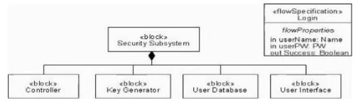
A user provides login credentials to the User Interface, and the Controller passes this information to the User Database The User Database in turn validates the user name and password (typed by PW In the «flow Specification») and responds with a Boolean value indicating whether the login was successful. The Controller provides the password to the Key Generator if login was successful.
