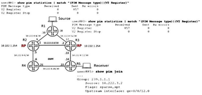
The source is currently sending multicast traffic using group 239.1.1.1 and R3 is receiving PIM register messages, but R2 does not have active source information.
