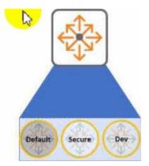
Aruba CX 6300 switch has routes in three different VRFs as per the example above. The user needs to leak routes between VRF Secure and VRF Dev. and also between VRF default and VRF Dev The customer Is not able to establish routing between directly connected networks 10.100.50.0/24 and 10.102.26.0/24.
