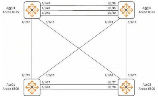
An engineer has attempted to configure two pairs of switches in the referenced configuration It is required to implement VSX at the aggregation layer
