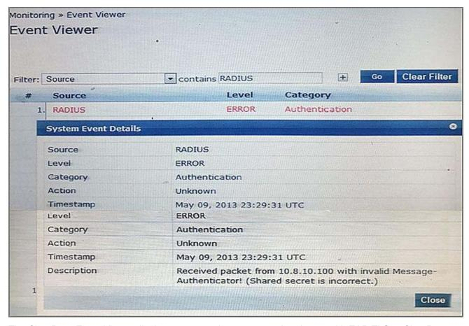
The ClearPass Event Viewer displays an error when a user authenticates with EAP-TLS to ClearPass through an Aruba Controller Wireless Network.
