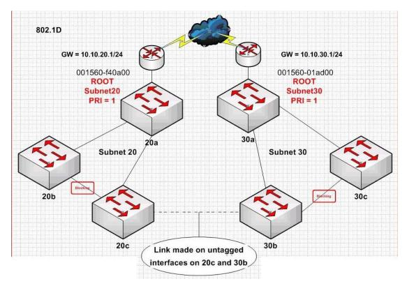
A user adds an untagged link between switch 20c and 30b. Which link transitions are blocked on subnet 20?
