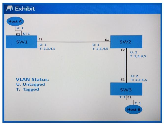
The exhibit shows a Layer 2 network between Host A (a Desktop Computer running Windows 7) and Host B (another Desktop Computer running Windows 7) and the list of VLANs Untagged (U) and Tagged (T) at each Ethernet interface: Host A transmits an Ethernet frame untagged on VLAN 1.
