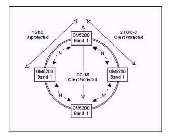
A. The design is well suited to the application because it offers electrical regeneration at each site to reduce amplifier requirements.
