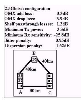
A. 28.87 dB; (There is no need for an amplifier because the un-amplified optical link budget is not exceeded.)
