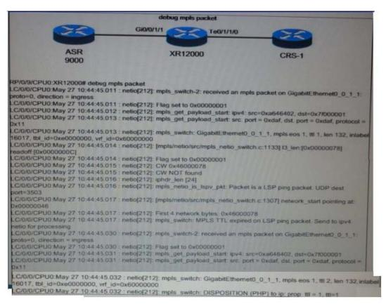
The output from the debug command is from the Cisco XR12000 series Router, which statement is true?
