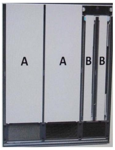
A. Block A, power supply. Block B is a supervisor module
