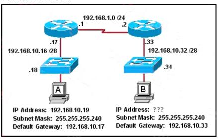
Host B has just been added to the network and must acquire an IP address.
