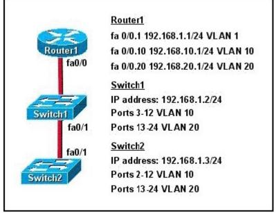
How should the FastEthernet0/1 ports on the 2950 model switches that are shown in the exhibit be configured to allow connectivity between all devices?
