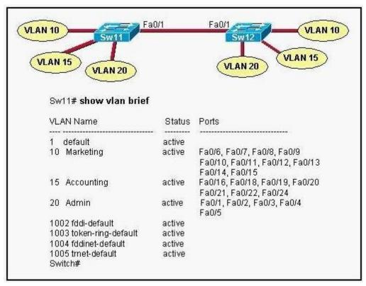
A.The Fa0/1 port is not operational on one of the switches.
