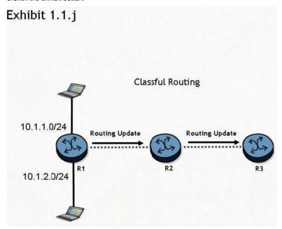
Routers R1 , R2, and R3 are running a classful routing protocol between them. Assuming that router R1 advertises all directly connected networks, how will these networks be
