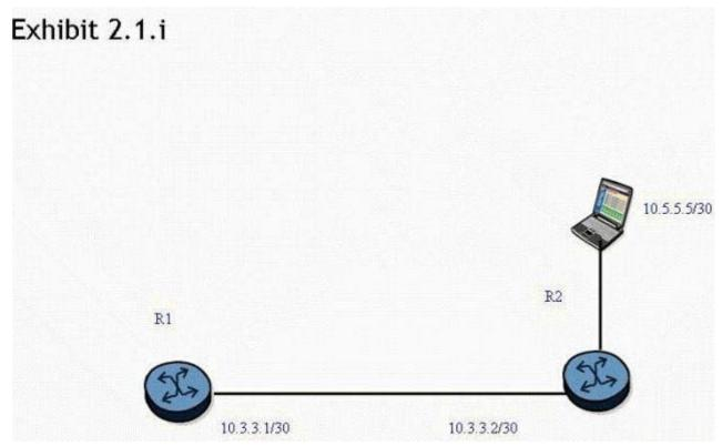
A static route is created on router R1 "using the "static-route 0.0.0.0/0 next-hop 10.3.3.2" command. What command can be used to test the static route on an Alcatel-Lucent 7750 SR?
