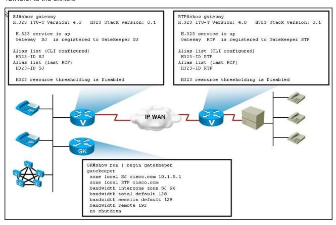
How many simultaneous G.729 calls can be established between sites SJ and RTP?
