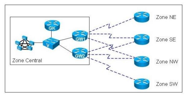
Which gatekeeper mechanism prevents the gatekeeper from using all the resources on either gateway 1 or gateway 2 when sending calls to zones SE and NW?
