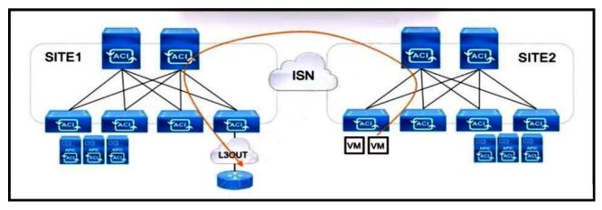
An engineer is configuring a production Multi-Site solution to provide connectivity from EPGs from a specific site to networks reachable through a remote site L3OUT. All required schema and template objects are already defined.
